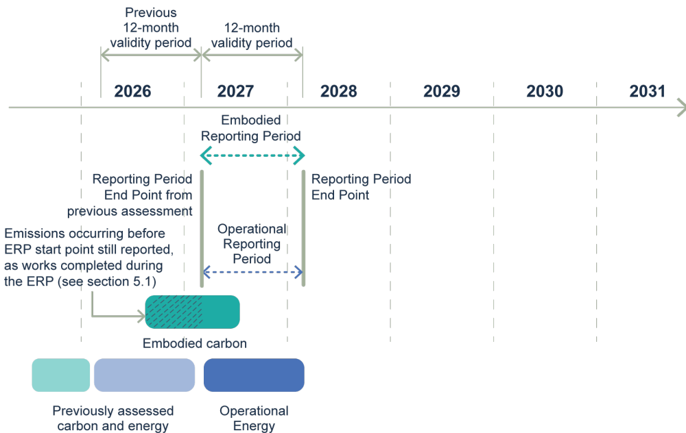
Figure 3 Typical RPEP, ERP and ORP for a second assessment, reporting and verification of a building. Note that the ERP for the second assessment starts the day after the previous RPEP.
